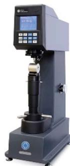
The test is performed by applying a specified sphere with force to the prepared surface. The width of indentation diameter specifies the hardness.
